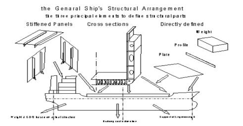
Normally only additional structures defined as panels and girders has to be added to cross sections to complete the model of the whole ship structure.
